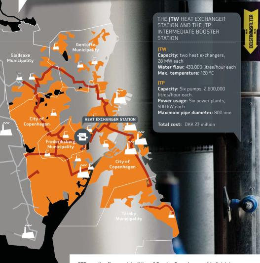
**CTR supplies five municipalities of Greater Copenhagen with district heating: Frederiksberg, Gentofte, Gladsaxe, Copenhagen and Tårnby.** CTR's transmission system comprises a 54-km distribution grid with 3 pump stations, 14 peak load stations and, finally, 26 heat exchanger stations that transfer the heat to the local district heating systems.
